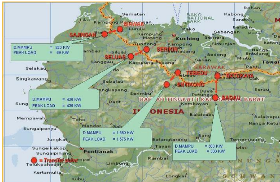
Figure 2 ASEAN Power Grid Indonesia – Malaysia
